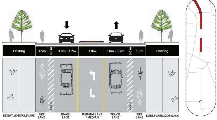
Figure 8.5 | Conceptual Shelbourne Street cross section, Christmas Avenue to Garnet Road and north of McKenzie Avenue to Torquay Drive
