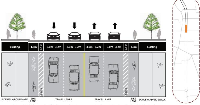
Figure 8.7 | Conceptual Shelbourne Street cross section, Garnet Road to North of McKenzie Avenue
